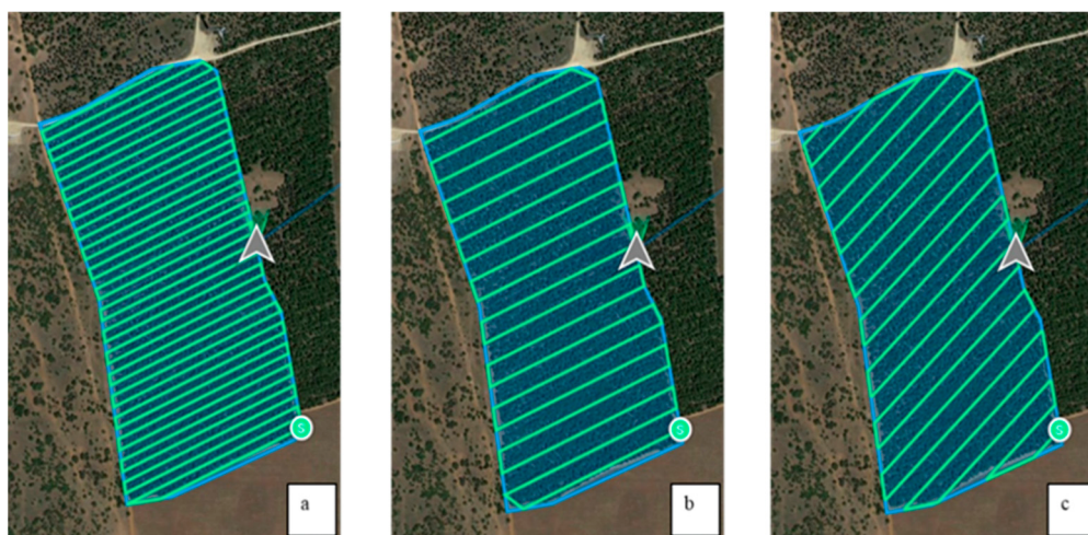
Figure 6. Drone routes; (a) 80% front and side overlap flight with 245^\circ angle ( 80 \times 80 F), (b) 80% front and 60% side overlap cross flights ( 80 \times 60 CF) with 245^\circ and (c) 225^\circ angles.
