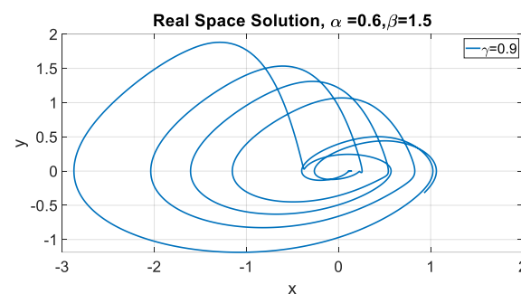
Figure 6. The real-space solution (projection in the x-y plane) of the \Lambda -fractional Chua system with parameters \alpha = 0.6 , \beta = 1.5 , and fractional order \gamma = 0.9 .
