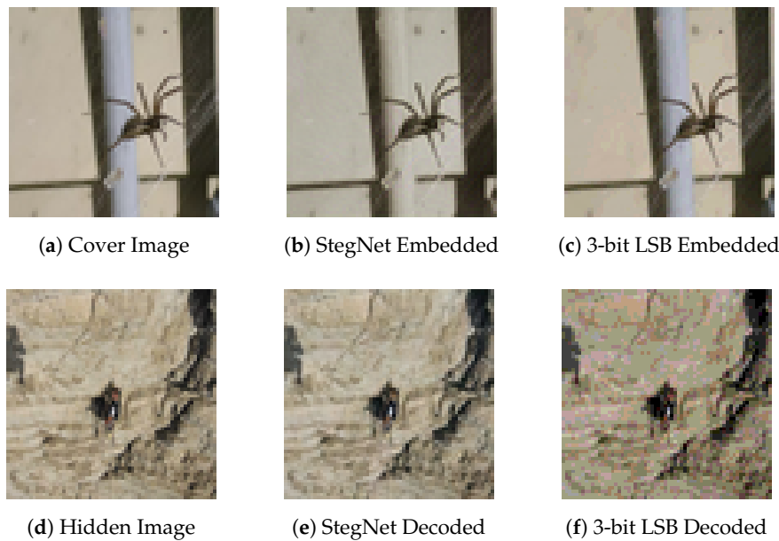
Figure 2. StegNet and 3-bit LSB Comparison Embedded-Cover-Diversity = 0.76%, Hidden-Decoded-Diversity = 1.8%, Payload Capacity = 23.57 bpp.
