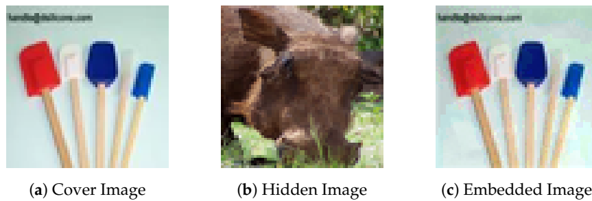
Figure 1. Vague Outline Visible in 4-bit LSB Steganography Embedded-Cover-Diversity = 50%, Hidden-Decoded-Diversity = 50%, Payload Capacity = 12 bpp.
