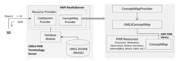
Figure 8. Architecture of UMLS FHIR terminology service.
