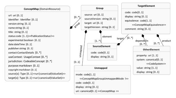
**Figure 4.** Using the UML class diagram to represent FHIR ConceptMap. The classes and attributes represent entities in the FHIR ConceptMap.
