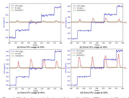
**Figure 4.** SSA detection on single miner violation with additive CPU usage. (**a**) One single miner increases 20% CPU usage at each time point; (**b**) One single miner increases 30% CPU usage at each time point; (**c**) One single miner increases 40% CPU usage at each time point; (**d**) One single miner increases 50% CPU usage at each time point.
