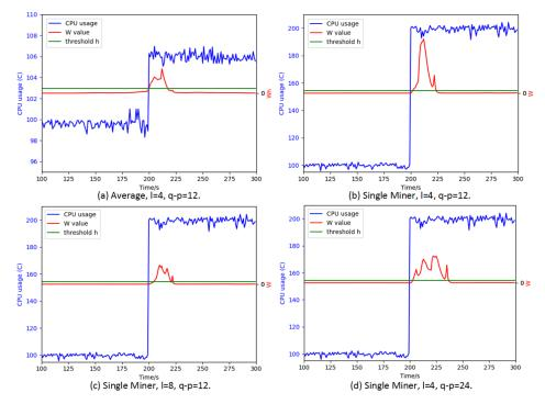
**Figure 3.** SSA detection on single miner violation with different parameter combinations. (a) Network level observation at the fog server; (b) Observation on a single miner; (c) Impacts of increasing *l* from 4 to 8 with the same matrix size; (d) Impacts of increasing the matrix size to 24 while maintain l = 4.
