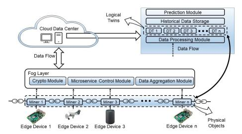
Figure 1. Illustration of MinT system architecture.
