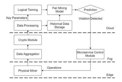
Figure 2. Miner twin-based fair-mining flowchart.
