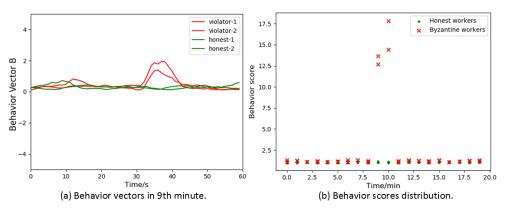
**Figure 5.** Behavior score distribution with sequential time spots. (a) The behavior vector from dishonest workers (red) varies from honest ones (green) when the byzantine workers gain more computing power; (b) Comparison between consensus scores associated with the byzantine nodes (red) and the honest nodes (green).
