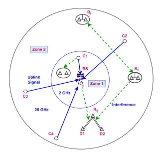
Figure 1. System model representing interference acting on D2D users.
