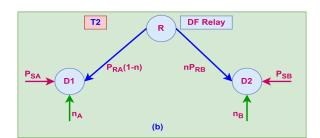
**Figure 2.** Line diagram representing the bidirectional exchange of information between *D*1 and *D*2 through the DF relay in the presence of interference and noise in different time slots. (**a**) time slot *T*1 and (**b**) time slot *T*2.
