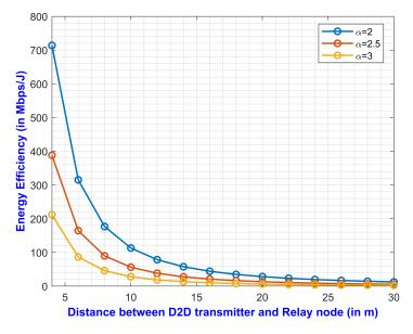
**Figure 5.** EE vs. distance between the D2D transmitter and the relay node for varying path loss exponents.
