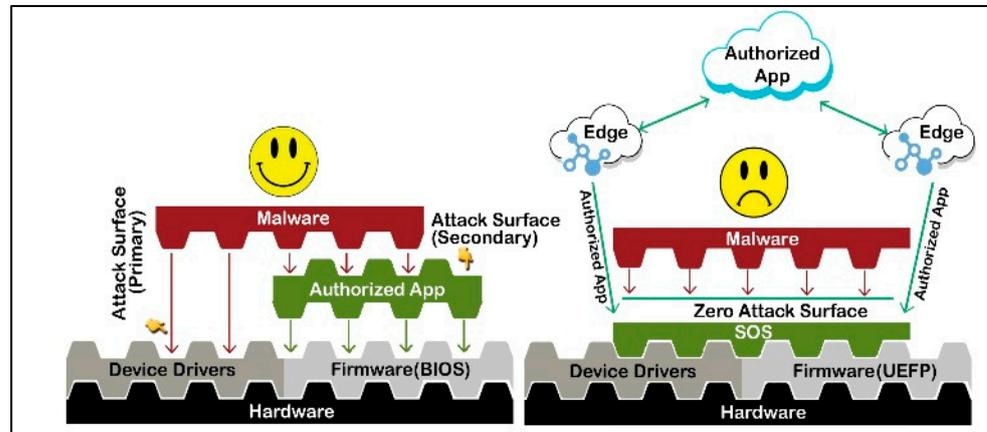
**Figure 5.** Comparison of architectural constructs of 3rd party permissions and attack surface between legacy IoT systems and ZVC.
