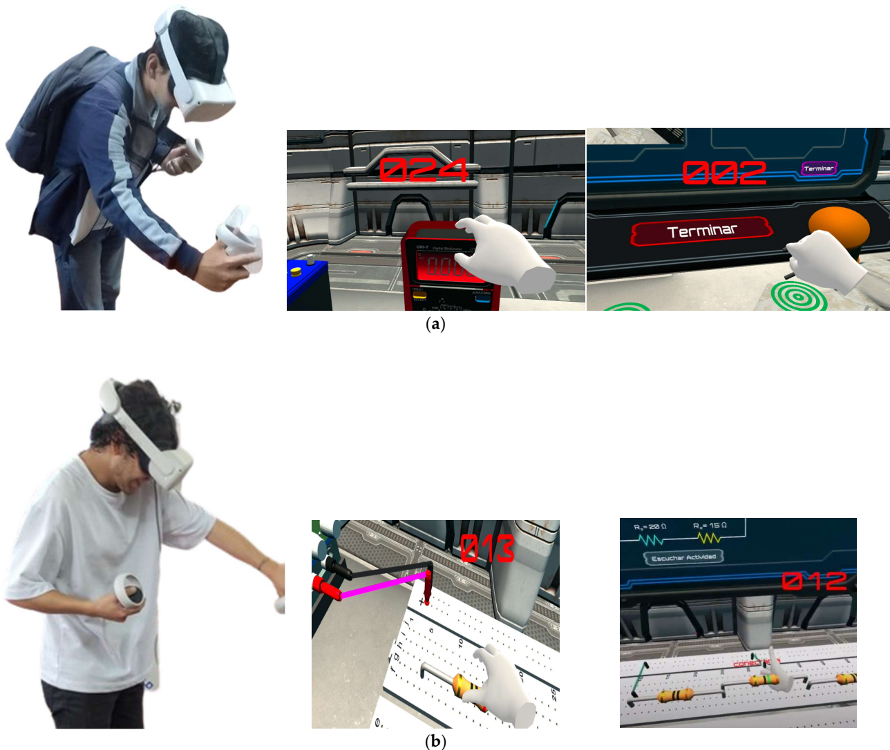
Figure 7. (a) Interaction with 3D objects for categorizing circuit elements. (b) Construction of a series circuit on a giant breadboard in the 3D virtual environment.
