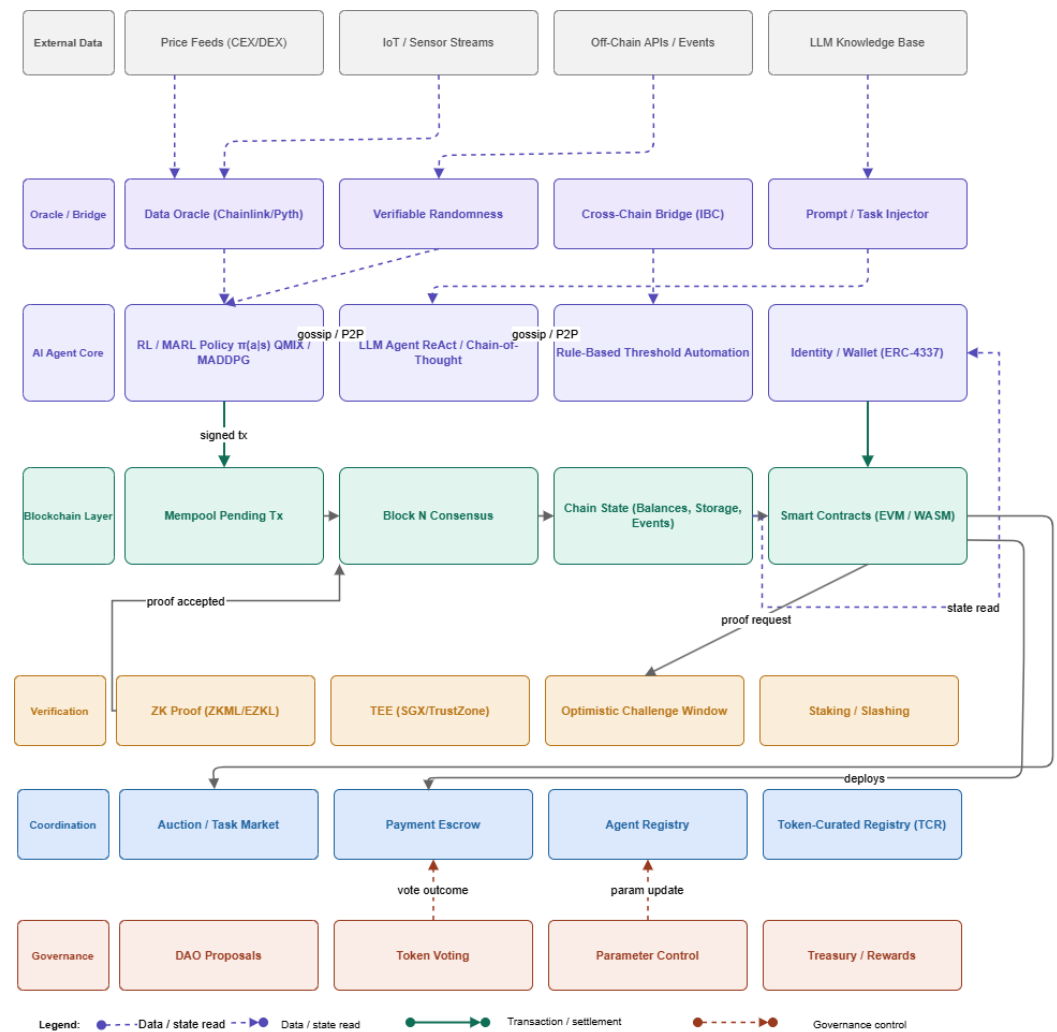
Figure 2. High Level architecture of a decentralised AI agent system across six layers: external data, oracle/bridge, AI agent core (RL/MARL, LLM, rule-based, ERC-4337), blockchain, verification, and coordination/governance. Dashed blue arrows = data reads; solid green = transaction settlement; dashed coral = governance control.
