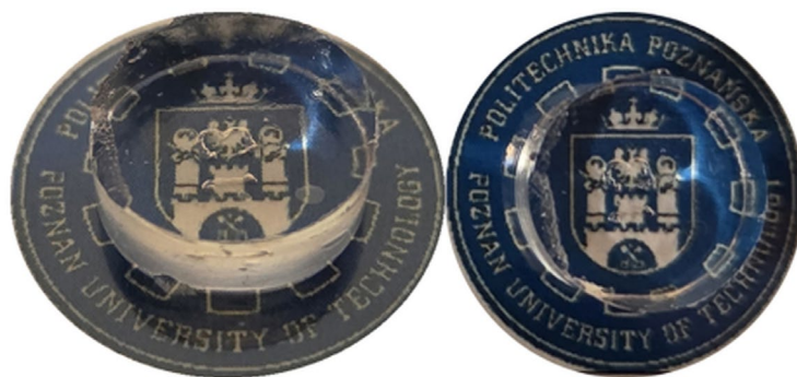
Figure 8. Photographs of the transparent hydrogel polymer electrolyte (HPE) containing 85 wt% aqueous choline lactate solution, demonstrating its homogeneous structure and absence of visible electrolyte leakage.
