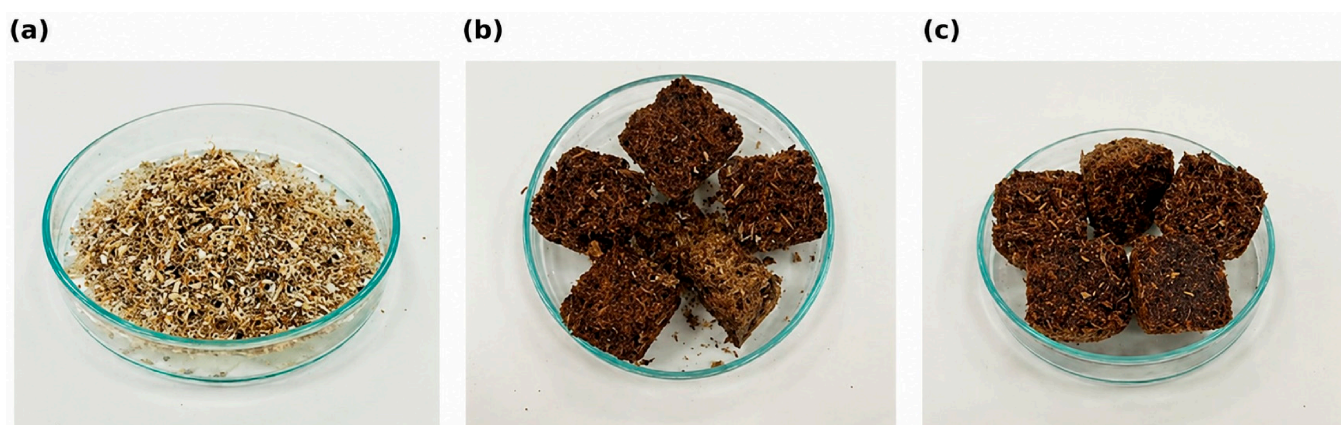
Figure 4. Representative macroscopic appearance of (a) untreated milled rapeseed straw and rapeseed-derived citric-acid-modified biogels prepared using (b) 180 mL and (c) 250 mL of 10 wt.% citric acid solution per 12 g of dry feedstock.
