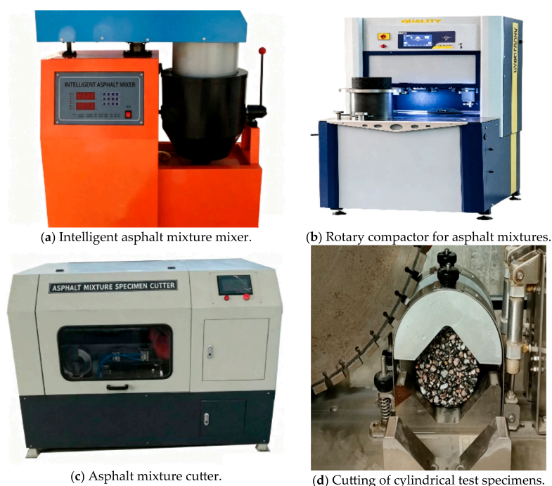
Figure 10. Molding and cutting of test specimens.
