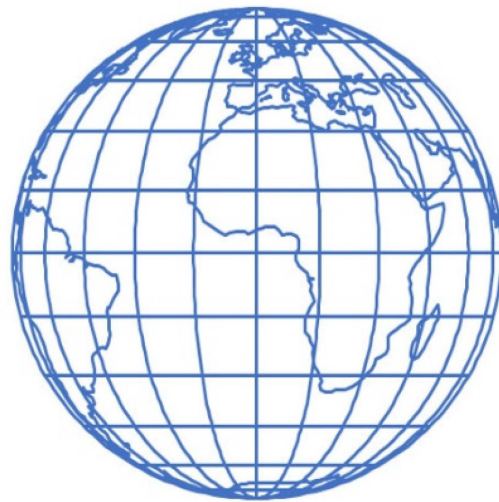
Figure 2. A hemisphere in the transverse orthographic projection.
