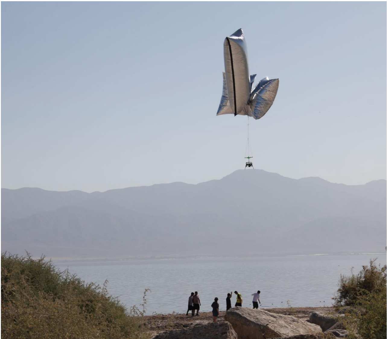
Figure 2. A balloon mapping rig flying above the North Shore of the Salton Sea shown with a picavet holding a GoPro7 and suspended by three mylar sleeping bag balloons.
