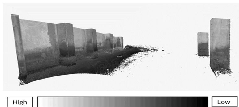
Figure 25. Scan data of the end pier of the highway bridge, Little Lake Worth, Florida (display by intensity) [29] (used with permission).
