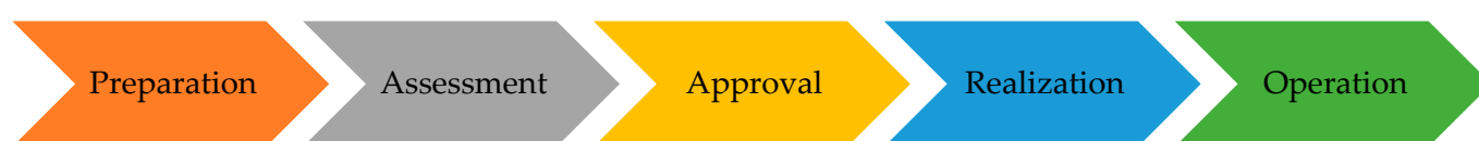
Figure 4. Schematic diagram of the small hydropower plant design process.
