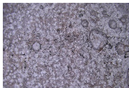
(f) C50X after 200 freeze-thaw cycle
