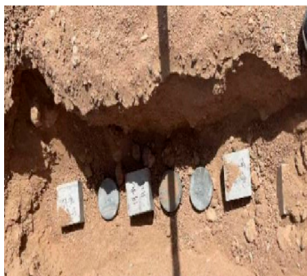
Figure 2. Outdoor experiments of specimens in 6% sulfate saline soil.
