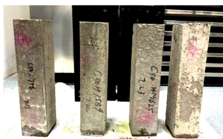
(c) Specimens after 100 indoor salt freeze-thaw cycles
