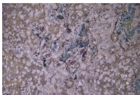
(e) C50N after 200 freeze-thaw cycles
