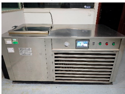
(c) Sulfate dry wet cycle test
