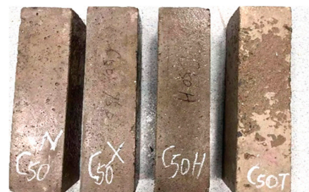
(b) Specimens after 50 indoor salt freeze-thaw cycles
