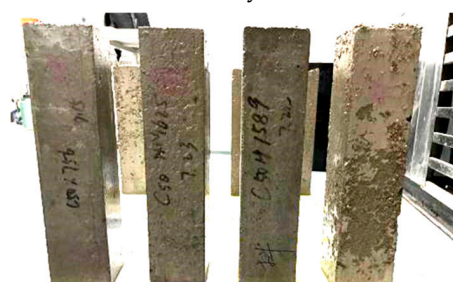
(b) Specimens after 50 indoor salt freeze-thaw cycles
