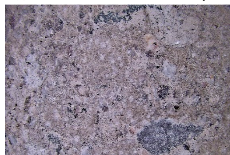
(h) C50H after 200 freeze-thaw cycles
