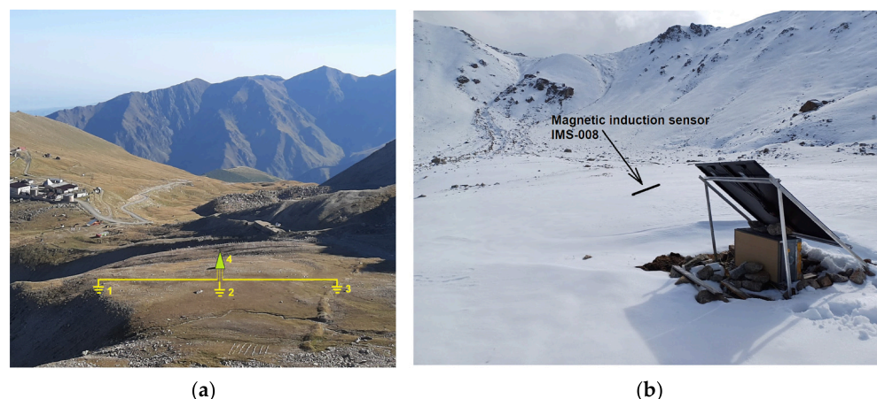
Figure 1. Experimental setup of the telluric current measurement system (a) and the IMS-008 induction-type magnetic sensor (b) for the registration of ultra-low-frequency (ULF) electromagnetic signals. 1 and 3—grounding electrodes for measuring telluric current variations, placed 120 m apart; 2—reference electrode; 4—measuring station [43.03692° N, 76.94230° E].
