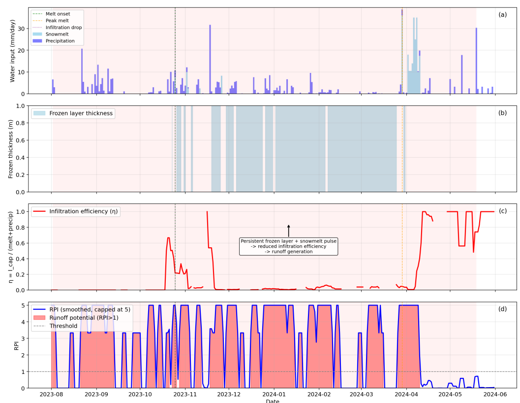
Figure 4. Coupled hydrothermal evolution at the Sergeevka station (North Kazakhstan region) during the 2023–2024 cold season: (a) water input (snowmelt and precipitation), (b) frozen layer thickness, (c) infiltration efficiency, (d) runoff potential index (RPI). Vertical dashed lines indicate key transition dates: green – onset of snowmelt, orange – peak snowmelt. The horizontal gray dashed line in panel (d) indicates the runoff potential threshold ( RPI = 1 ).
