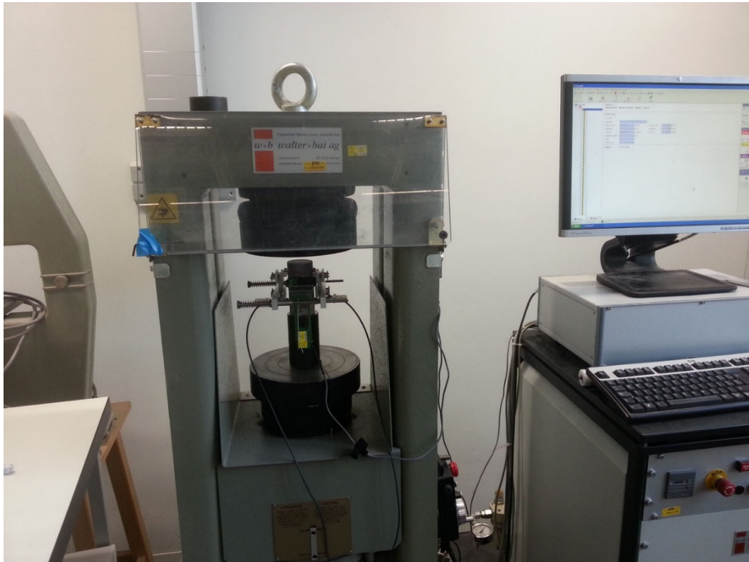
Figure 3. Deformation-controlled test setup used for uniaxial compressive tests at ETH Zürich in 2015 (Photo taken by Ömer Ündül).
