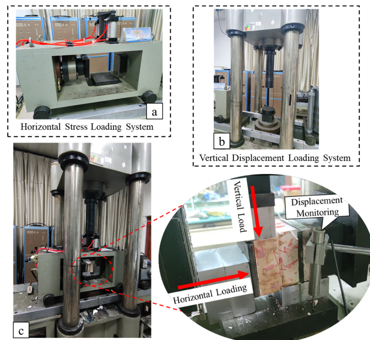
Figure 5. Test system and loading method. (a) Horizontal loading system for applying normal stress to the rock joint. (b) Vertical loading system for inducing rock joint dislocation. (c) RLJW-2000 machine and close-up of the bolt-joint configuration within the shear box.
