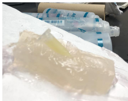
Figure 1. Urate suspension in Eppendorf on bed of ultrasound gel for imaging.
