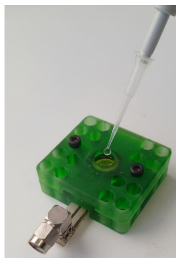
Figure 7. Batch-mode operation using distilled water. The sample is deposited directly onto the crystal using a micropipette, without circulation. Once the active area of the crystal is fully covered, the measured f_r and D are independent of the total deposited sample volume [22,23].
