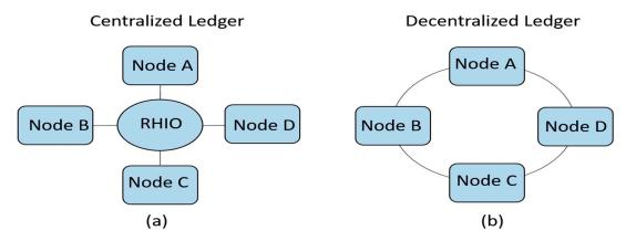
**Figure 1.** Centralized vs. decentralized system. In (a), there are multiple ledgers but all records are held in RHIO, whereas in (b), there is only one ledger but every node has some level of access to that ledger. The decentralized architecture removes the need for trusted third party, makes transactions faster, and removes the transaction fees charged by the trusted third party (RHIO).
