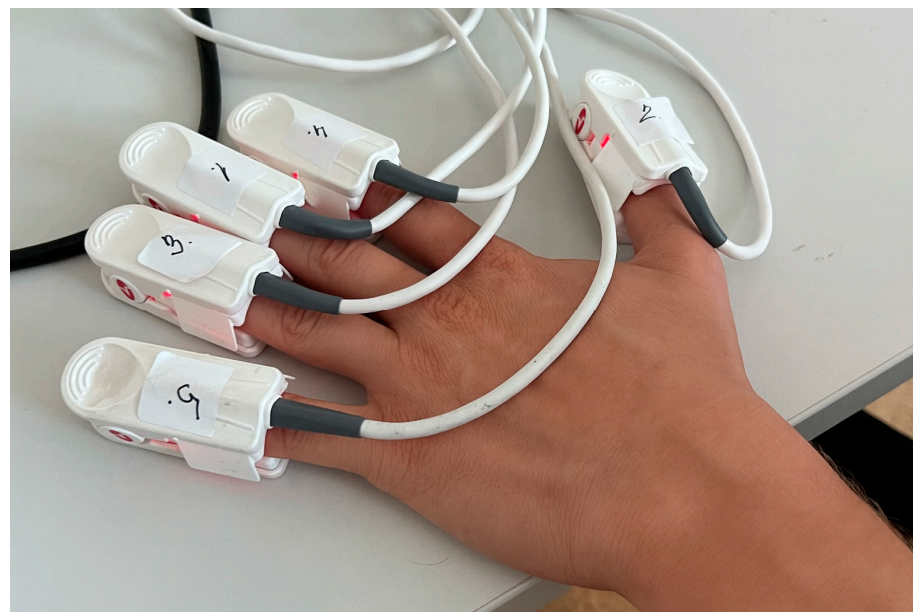
Figure 1. Placement of finger sensors. Masimo Radical-97 (LNCS DCI) sensors were randomly assigned and placed on each finger of the left hand. The participant was seated with the left hand resting still on the table, wrist and palm facing down.
