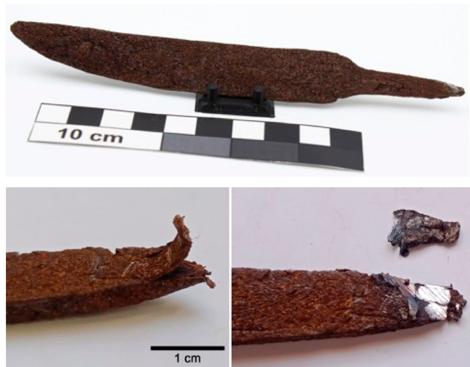
Figure 2. The blade dagger B analyzed in this study. (Top): full-size image. (Bottom): detailed images that exhibit the strongly oxidized rusty and weathered surface and the plate removed from the scaled tip of the blade.
