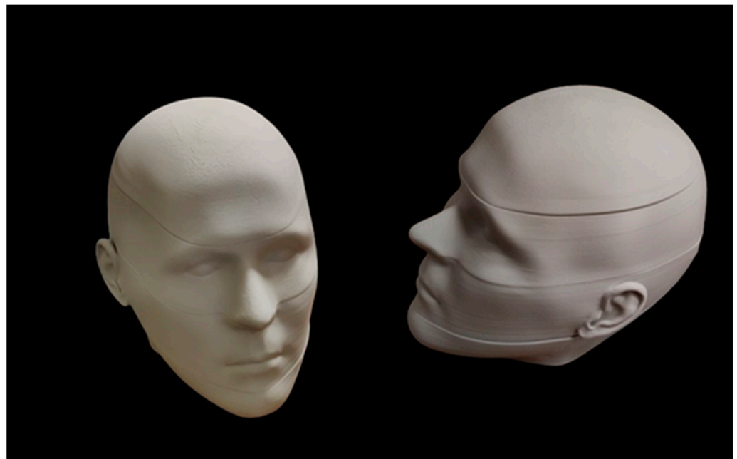
Figure 11. The figure depicts printed segments arranged to form a complete model that requires postprocessing of segment joints.
