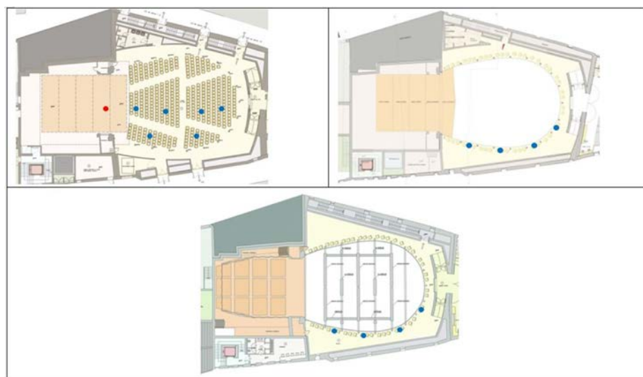
Figure 7. Source (red dot) and microphone positions (blue dots).
