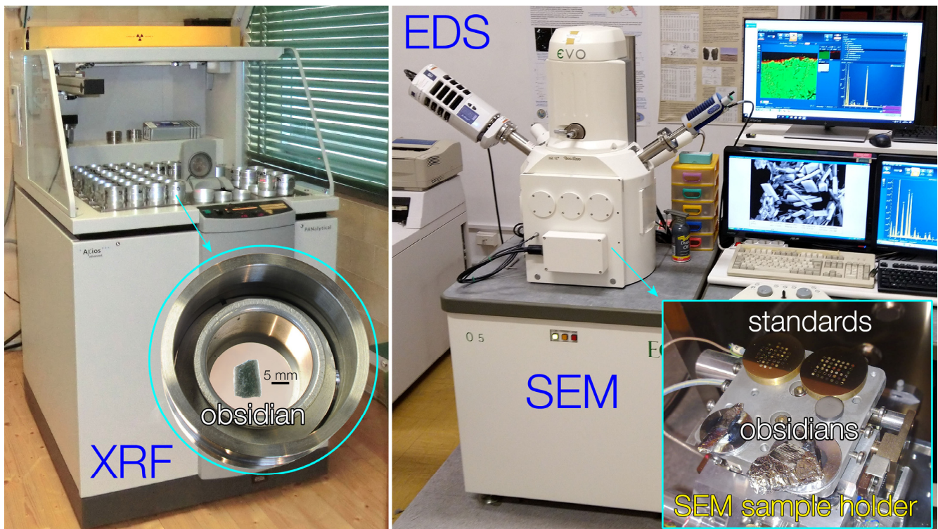
Figure 3. On the left, the X-ray fluorescence (XRF) spectrometer with detail of the sample holder (in the light blue circle) in which the obsidian specimen seems to be suspended in the air (see text for explanation); on the right, the scanning electron microscope (SEM) equipped with an energy-dispersive spectrometer (EDS) and a detail of the sample holder (in the light blue rectangle) on which are mounted the obsidian samples and the reference standards.
