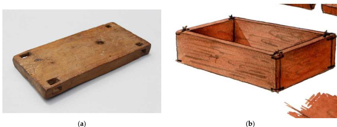
Figure 2. Piece that formed part of a pre-Hispanic adobe-making mould: (a) piece located in the Arturo Jiménez Borja Museum in the city of Lima [22]; (b) proposal of how the components of a pre-Hispanic adobe mould might have been joined together [23].
