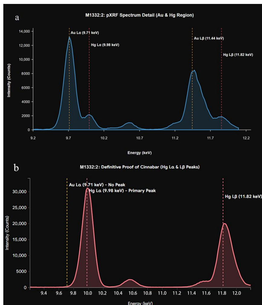
Figure 3. XRF spectra of the attachments on the painted mirror excavated from M1332 at the Yafubei cemetery, Linzi. (a) detailed pXRF spectrum of the gold-coloured applique highlighting Au and Hg peaks; (b) spectrum of the red pigment showing characteristic Hg peaks.
