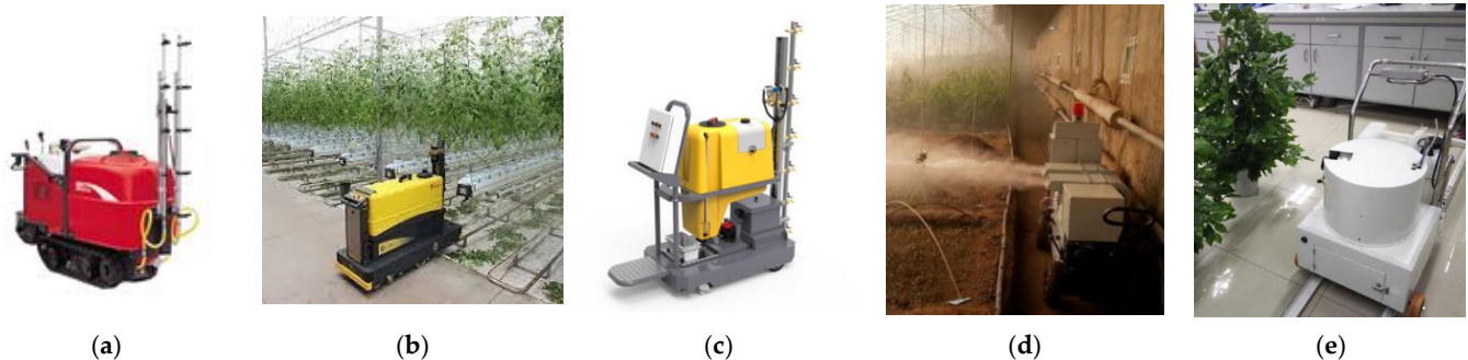
Figure 2. Major types of ground sprayers in greenhouses: (a) crawler self-propelled sprayer, (b) ground track sprayer, (c) self-propelled sprayer, (d) self-propelled ultrasonic atomizer, and (e) self-propelled mist sprayer.
