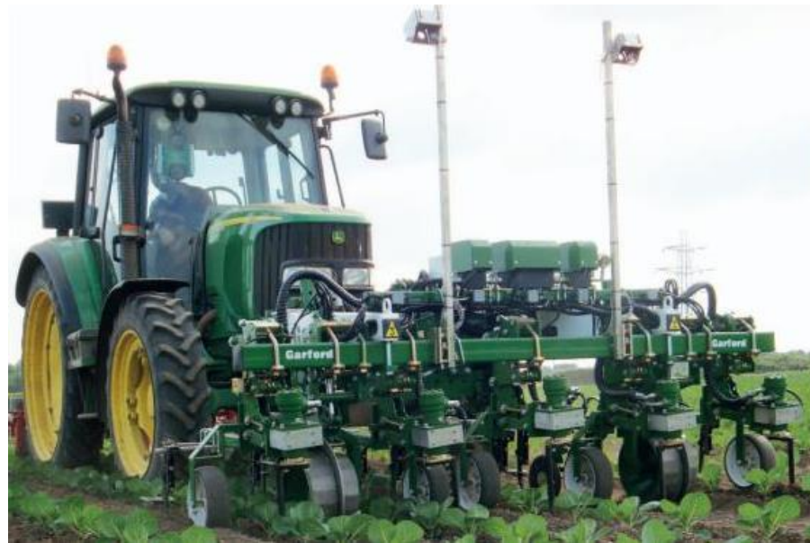
Figure 7. Rotary notched disc hoe weeder.
