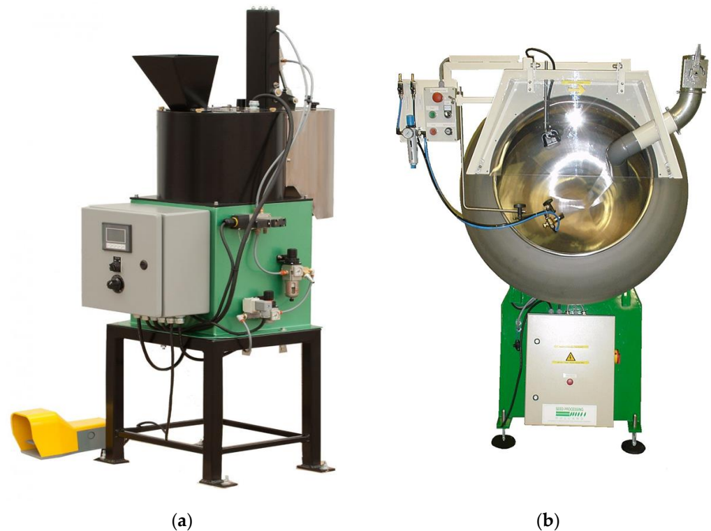
Figure 5. Major types of seed coater: (a) rotary seed coater, and (b) drum seed coater.
