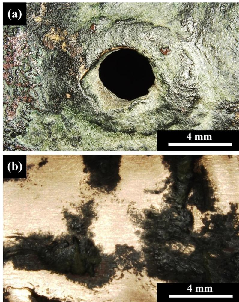
**Figure 6.** The copper-alloy tube multifocal LM observation, showing (a) the small drilled hole surrounded by a patina cover and some corrosion products on the back of the object and (b) the bright metal areas that were locally sanded (back of the object) before performing the XRF analysis of the core metal; the dark areas are the remains of oxides and corrosion products.
