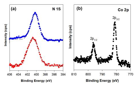
**Figure 6.** (a) High-resolution XPS spectra of N1s for Im-EtPMO (red line) and Im-EtPMO-Co (blue line). (b) High-resolution Co2p XPS spectrum for Im-EtPMO-Co.
