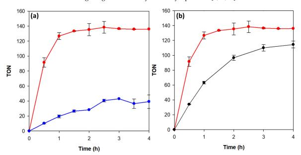
**Figure 7.** (a) Photocatalytic HER with Im-EtPMO-Co (red line) and  $Co(dmgH)_2(Im)Cl$  homogeneous catalyst (blue line). (b) Photocatalytic HER with Im-EtPMO-Co (red line) and py-etPMO-Co (black line) as catalysts.
