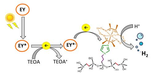
**Scheme 2.** Schematic representation of photocatalytic hydrogen evolution reaction with TEOA and Eosin Y (EY) as electron donor and photosensitizer, respectively. (EY\*, photoexcited EY).
