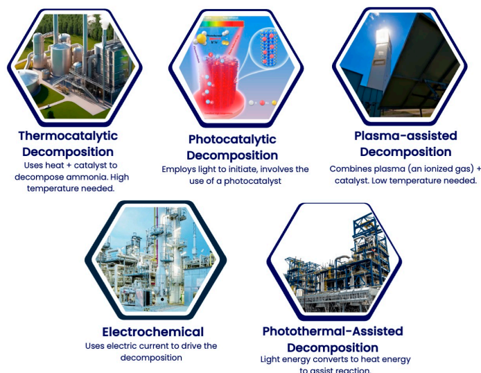
Figure 1. Types of Ammonia Decomposition comprising Thermocatalytic Decomposition, Photocatalytic Decomposition, Plasma-Assisted Electrochemical, and Photothermal-Assisted.
