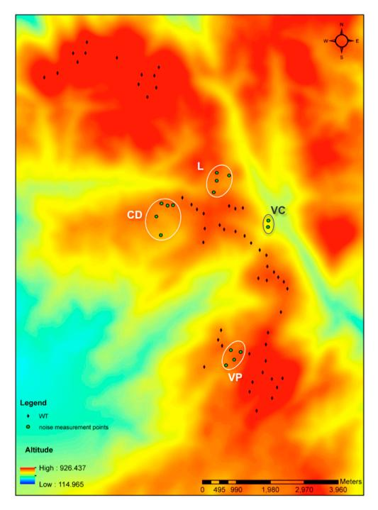
**Figure 2.** Map of the wind farm studied with the corresponding measurement locations (black dots: Wind Turbines; green circles: dwellings at the measurements' locations, L: Lagoa, CD: Campo Dianteiro, VC: Várzea Cova, VP: Vila Pouca).
