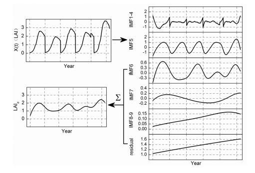
**Figure 3.** Rationale for extracting heavy metal stress signal based on ensemble empirical mode decomposition (EEMD). The LAI time series is broken down into nine modes and a residual that are divided into three main components: other short-term stress (IMF1-4), the crop inherent growth trend (IMF5), and heavy metal stress (IMF6-residual). LAI: Leaf Area Index; IMF: Intrinsic Mode Function.
