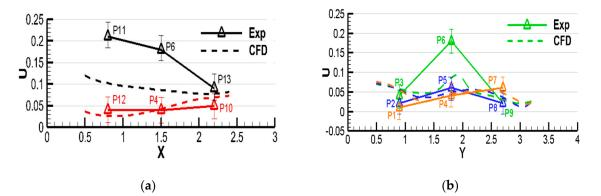
**Figure 4.** Comparison between experimental measurements and computational results for case A ((a): along the x-axis, (b): along the y-axis. The same color represents the same location, Exp: Experiment, CFD: computational fluid dynamics).
