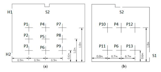
Figure 2. Detailed locations of the measurement points: (a) Plane X = 1.5 m; (b) plane Y = 1.8 m.
