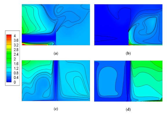
Figure 9.  $CO_2$  concentration cloud map of Y = 1.5 m section: (a) Case 1, (b) case 2, (c) case 3, (d) case 4.
