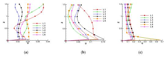
**Figure 12.** Velocity distributions along different lines in the center of subzones in Model II: (a) Down-supply up-return; (b) floor-supply up-return; (c) top-supply down-return.
