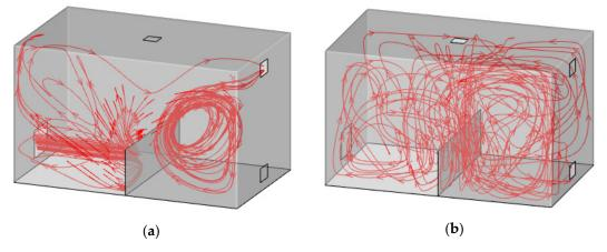
**Figure 8.** Streamlines under two ventilation patterns in Model I: (**a**) Down-supply up-return; (**b**) top-supply down-return.
