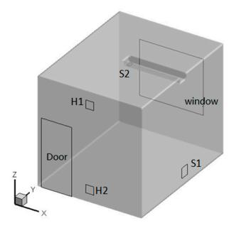
Figure 1. Schematic diagram of the test chamber.
