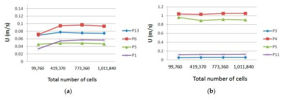
Figure 3. Results of grid independent test. (a) Case A; (b) case B.
