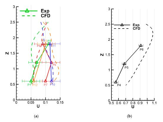
**Figure 5.** Comparison between experimental measurements and computational results for case B ((a) and (b) were along the z-axis, which passed different measurement points. The same color represents the same location, Exp: Experiment, CFD: computational fluid dynamics).
