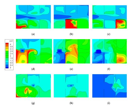
**Figure 13.** Distribution of CO<sub>2</sub> concentration at the height Z = 0.75 m: (a) Case 9, (b) case 10, (c) case 11, (d) case 12, (e) case 13, (f) case 14, (g) case 15, (h) case 16, (i) case 17.
