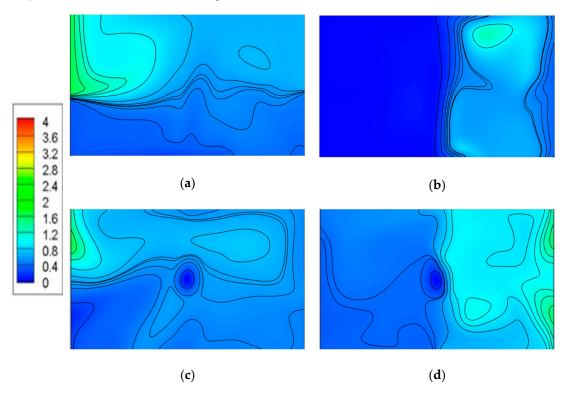
Figure 10.  $CO_2$  concentration cloud map of Z = 1.6 m section: (a) Case 1, (b) case 2, (c) case 3, (d) case 4.
