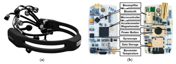
**Figure 3.** Emotiv Epoc helmet (**a**) and designed ECG holter (**b**).
