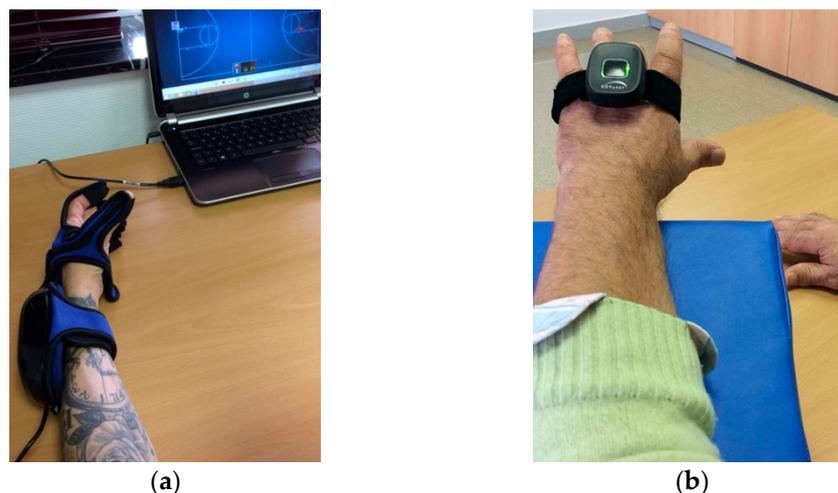
**Figure 1.** (a) HandTutor© glove (flexion–extension of the fingers); (b) 3DTutor© (wrist extension).
