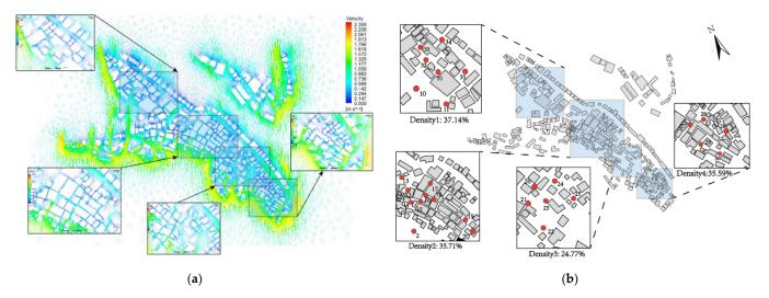
Figure 5. (a) Wind environment of study case. (b) Study cases are divided by different building densities.
