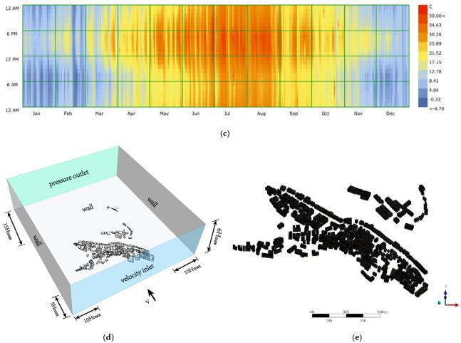
Figure 3. (a) Distribution of measuring points. (b) Scope of the study case. (c) Outdoor temperature distribution of study cases throughout the year. (d) Study case boundary conditions. (e) Meshing of study cases.
