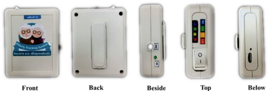
Figure 4. The external appearance of the tracking device.
