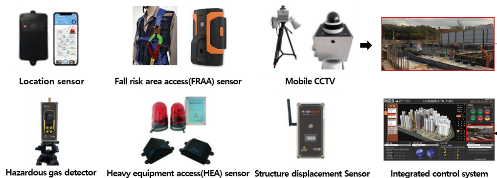
Figure 7. Types of SCSTs used in the test beds.
