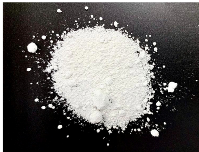
Figure 1. Reagent-grade \text{TiO}_2 powder (anatase, 99% purity).
