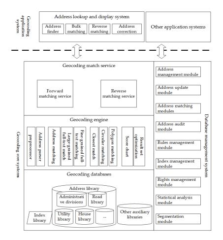
Figure 8. Architecture of the geocoding service system.
