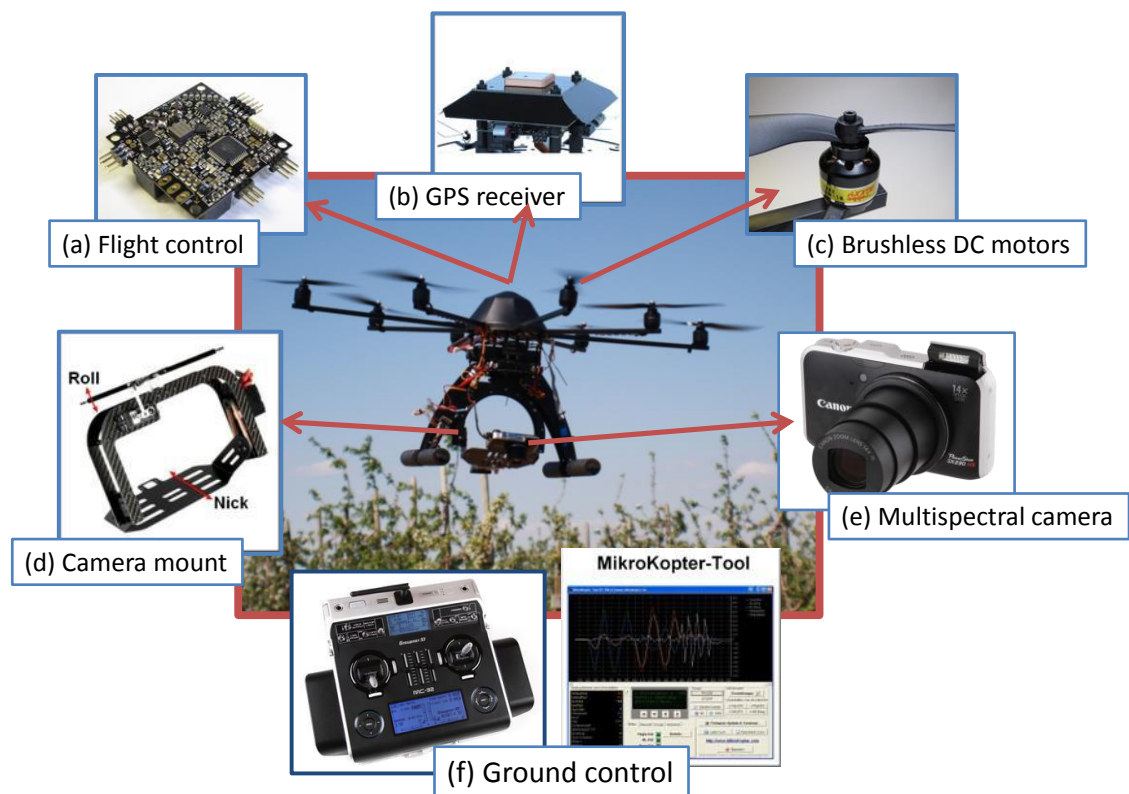
Figure 3. Unmanned aerial vehicle with multispectral camera (vegetation stress camera).
