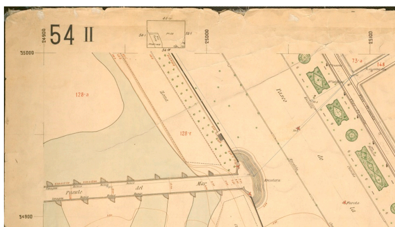
Figure 2. Grid frame corner of the map number 54 II. The X axis and the Y axis show the local coordinates, on this image from 24,900 to 25,100 m and from 35,000 to 34,900 m respectively.
