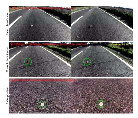
**Figure 4.** Examples of images captured by the MMS2 during real surveys: in the two upper images, the algorithm failed to detect the WVC (failed classification); in the middle images, the algorithm correctly detected the WVC (correct classification); and in the lower ones, the algorithm detected an animal incorrectly (false positive). The ZED camera is a dual-camera, always providing two images with slightly different angles.
