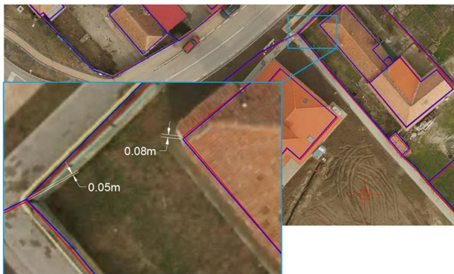
**Figure 15.** Comparison of the recorded boundaries using the proposed procedure (in blue) with those obtained from the official Cadastral Maps.
