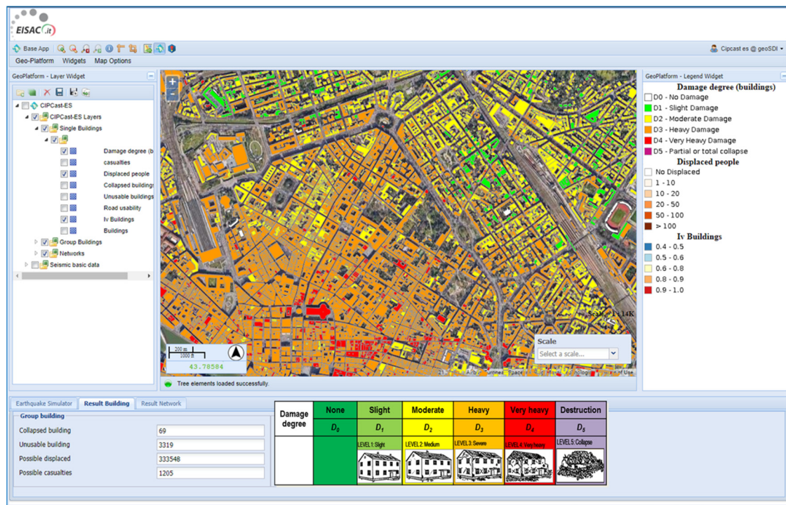
Figure 2. Assessment and representation of earthquake-induced physical damage in ARCH DSS.
